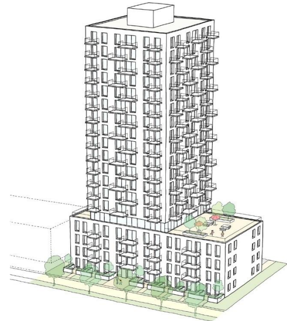
Figure 11.36 - Typical 20 storey apartment (axo)
