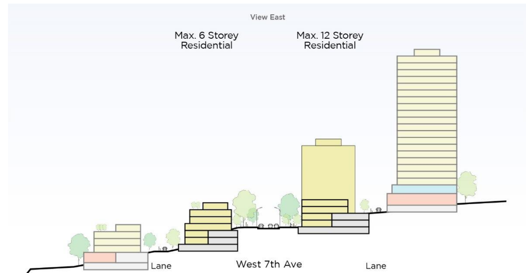
Figure 9.4 - Illustrative Street Section of West 7th Avenue between Alder and Spruce Streets
