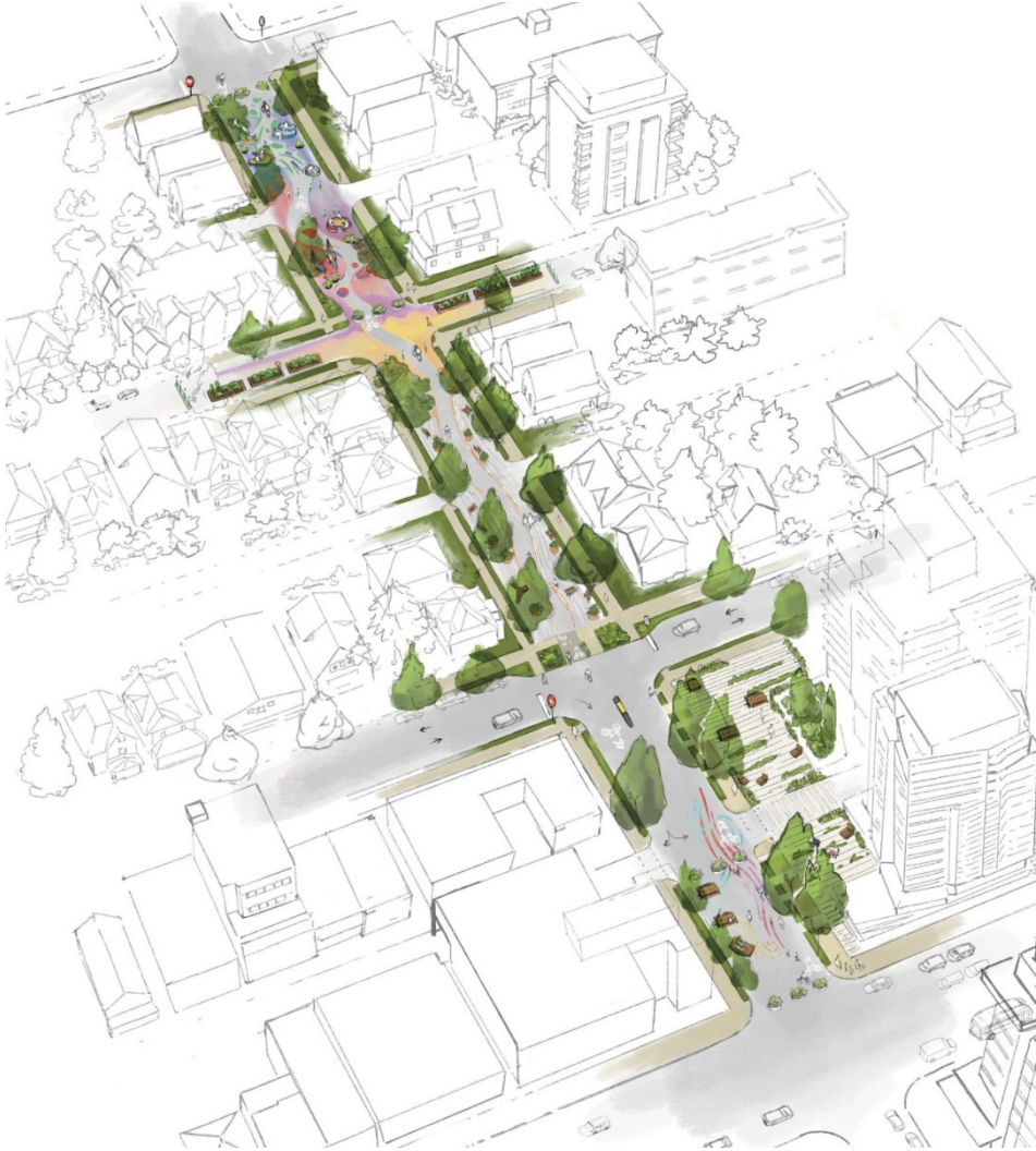
Figure 55: Example of a car-free street completed using temporary materials and without major reconstruction of the street
