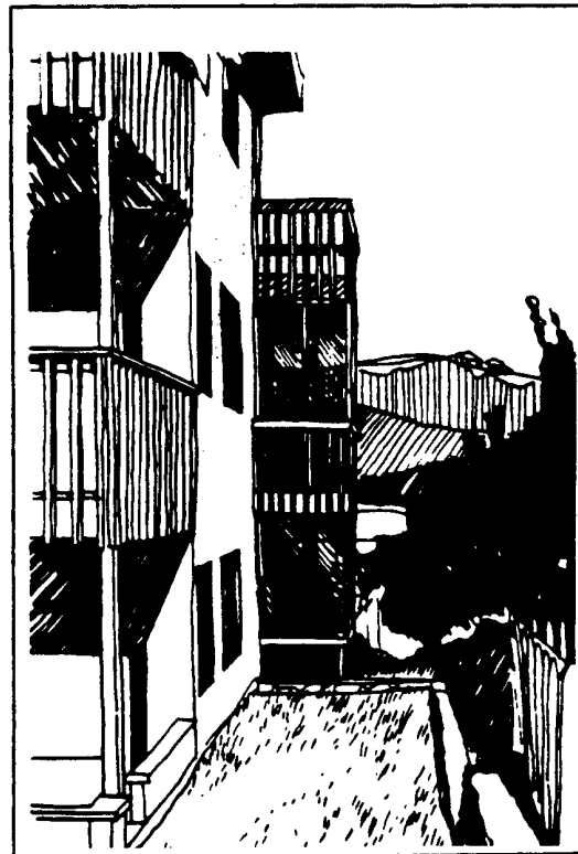
Figure 2. Example of Discouraged Enclosed Corner Blocking Views
