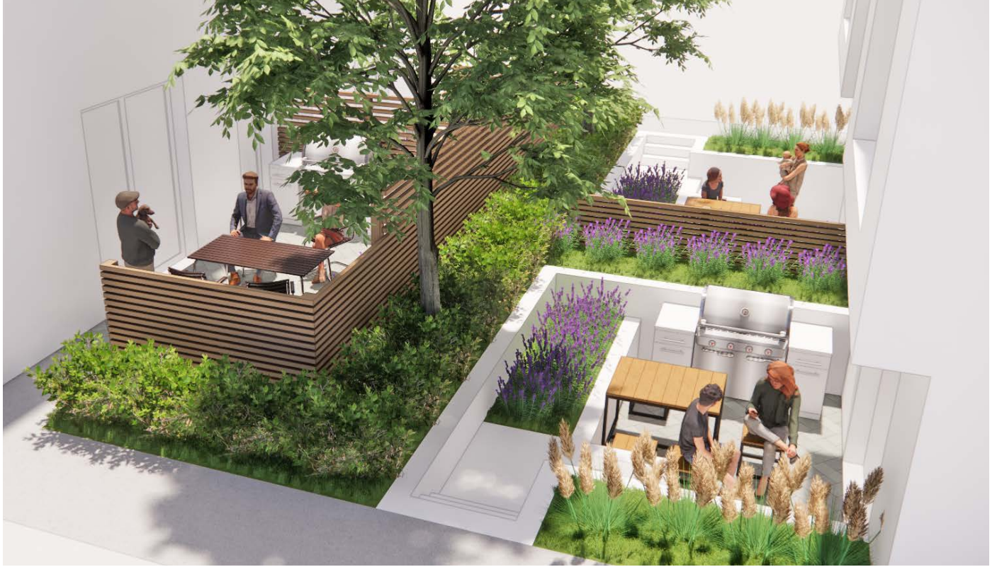
Figure 59: Managing grade change using a stepped wall or low wall with sloped planting will create desirable outdoor space for basement units.
