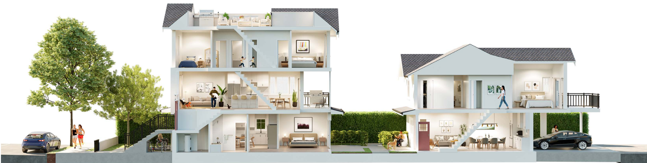
Section model of a multiple dwelling building with six units - four units in the front and two units in the rear in a courtyard configuration. Credit: Formwerks Architecture
